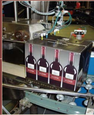
Automated machines apply the water-based adhesive while the pallet is being built.
