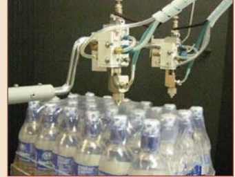
Automated machines apply the water-based adhesive while the pallet is being built.
